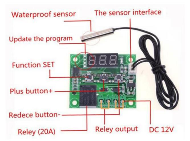
Connect the power supply and equipment, to the controller power supply, as measured temperature is displayed, press the SET button, the display temperature flashes, press "+" "-" to set the desired temperature
